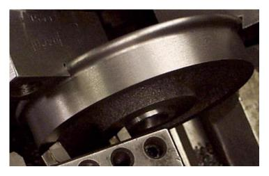
Third operation. Rim chamfering with brazed carbide tool bit mounted on tool holder mounted on lathe compound slide using manual cross feed. Spindle speed 370 rpm., 460 sfpm. After the right tool bit completes facing the front hub, the power cross feed is disengaged and the cross slide is fed manually to machine the rim chamfer with the left tool bit.
