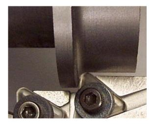
Second operation continued. After the carriage reaches the left side carriage stop, it is held there until the carbide insert no longer produces any chips. The carriage is then moved to the right to the previous starting position. Completion of the second operation produces the finished flange width. The compound slide dial reference "CP-A" controls the finished flange width and is adjusted in order to compensate for tool wear.
