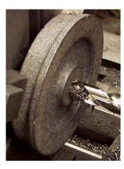
Third operation. Tandem facing of back of the flange and back hub with brazed carbide tool bits mounted on tool post mounted on lathe compound slide using lathe power cross feed. The cross slide is moved to a position where the outside tool bit will clear both the chuck jaws and the rough casting. The carriage is then moved to the left carriage stop and locked. The power cross feed is then engaged. Adjustment of the left carriage stop simultaneously controls the depth of cut of both tool bits.
