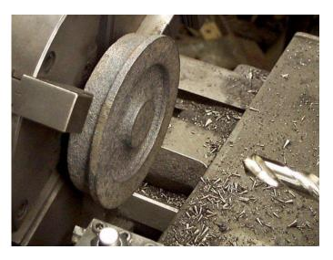
Second operation. Hole drilling with 21/32 inch diameter high speed steel "stub" twist drill mounted on turret. Spindle speed 370 rpm., 64 sfpm., turret hand feed.
