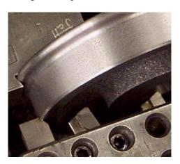
Fourth operation. The cross slide is moved approximately 0.100 inches from the work, the carriage is unlocked and moved approximately two inches from the work. The cross slide is then returned to the starting position for the first operation. The lathe is stopped and the completed wheel is removed. Third set up average production rate 55 wheels per hour.
