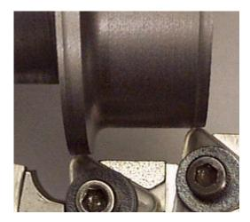
Third operation continued. When the right carbide insert nears the flange throat radius the power feed is disengaged and the carriage is fed manually to continue cutting the finished tread diameter. Manual feed rate is approximately 0.004 ipr. After the carriage reaches the left side carriage stop, it is held there until the carbide insert no longer produces any chips.
