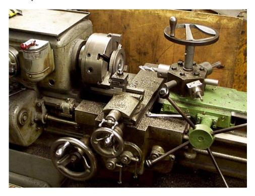
First operation. Mounting rough cast iron wheel blank on chuck and starting lathe.
