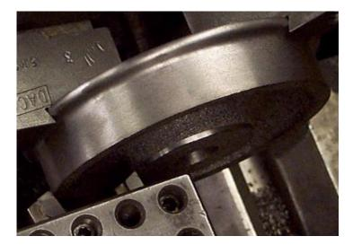
Second operation continued. Tandem facing of rim and front hub. Spindle speed 370 rpm., 460 sfpm. at the beginning of the middle tool bit cut, lathe power cross feed rate 0.003 ipr.
