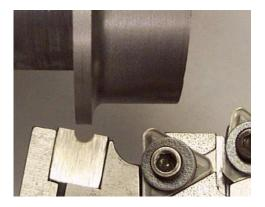
Forth operation continued. Three views showing the radius form tool at the beginning, middle and end of the cut. Spindle speed 100 rpm., 131 sfpm., manual cross slide feed rate approximately 0.004 ipr. The cross slide dial reference "CS-C" is adjusted in order to compensate for tool wear.
