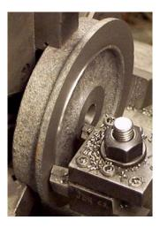
Third operation continued. After the outside tool bit completes facing the back of the flange the power cross feed and carriage lock are disengaged. The carriage is moved to the right and the cross slide is moved to bring the tool post back to the original parking position which clears the tool post and tool bits from the chuck jaws and the ram of the turret.
