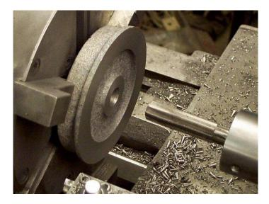
Fifth operation continued. The reaming operation produces the final hole diameter and maintains this diameter within close tolerances for each wheel produced.
