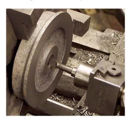
Forth operation continued. Boring bar at the end of the cut. After completion of the boring operation the boring bar is withdrawn and the turret is indexed from the boring bar to the reamer.
