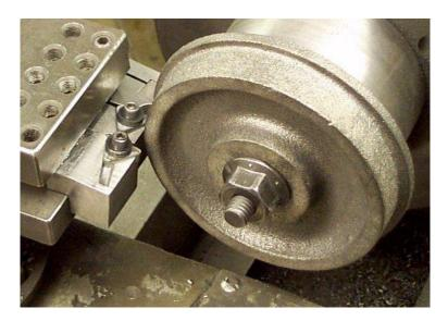
Second operation. Machining of first rough flange diameter of 4.920 inches, rough tread diameter of 4.520 inches and finished flange width of 0.156 inches. The compound slide dial is set to reference "CP-A," the carriage is positioned for starting the cut, the cross slide dial is set to reference "CS-A" and the power carriage feed is engaged.
