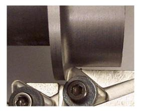
Third operation continued. The cross slide is moved to bring the tool bits away from the work. The carriage is then moved to the right side carriage stop.
