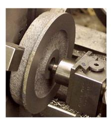
Fifth operation. Hole reaming with 3/4 inch diameter high speed steel "stub shank" reamer mounted on turret. Spindle speed 370 rpm., 73 sfpm., turret hand feed.
