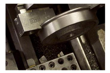
Second operation. Tandem facing of rim and front hub with brazed carbide tool bits mounted on tool holder mounted on lathe compound slide using lathe power cross feed. The carriage is moved to the left side carriage stop and locked and the power cross feed is engaged. Adjustment of the compound slide simultaneously controls the depth of cut of both tool bits.
