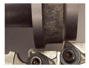
Second operation continued. When the right carbide insert nears the outside of the rough flange the power feed is disengaged. The carriage is then fed manually to simultaneously cut the outside of the flange and continue cutting the rough tread diameter. Manual feed rate is approximately 0.004 ipr. The right carbide insert is set to produce an 80 degree flange angle.
