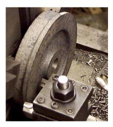
Third operation continued. The outside tool bit begins facing the back of the flange before the inside tool bit begins facing the back hub. Spindle speed 370 rpm., 494 sfpm. at the beginning of the outside tool bit cut, lathe power cross feed rate 0.003 ipr.
