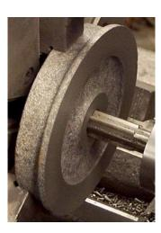
Sixth operation. After the reamer is withdrawn the turret is indexed from the reamer to the twist drill, the lathe is stopped and the wheel is removed. Average first set up production rate 16 wheels per hour.
