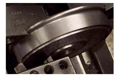
Second operation continued. The right tool bit continues facing the front hub after the middle tool bit has completed facing the rim. The tool bits are mounted in such a way that the cutting of the middle tool bit was begun and completed during the longer cut taken by the right tool bit.
