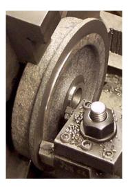
Third operation continued. The outside tool bit continues facing the back of the flange after the inside tool bit has completed facing the back hub. The tool bits are mounted in such a way that the cutting of the inside tool bit was begun and completed during the longer cut taken by the outside tool bit.
