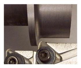
Forth operation. Machining of 0.094 inch flange radius and finished flange height of 0.188 inches. The carriage is locked against the right side carriage stop which is adjusted to bring the flange radius form tool into proper location with the compound slide dial setting remaining at reference "CP-B." The cross slide is manually fed into the work and is stopped when the cross slide dial reading reaches reference "CS-C."
