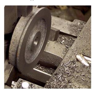
Second set up for turning operations to produce D&R Cylindrical Wheel Tread and Flange Contour having 4.500 inch diameter wheel tread, 3/32 inch flange throat radius, 5/32 inch flange width, 80 degree outside flange angle, 3/16 inch flange height and 3/32 inch flange radius on 13 inch "Sheldon" gear head lathe equipped with cross slide quick change tool post, multiple tool bit holder and wheel tread and flange turning fixture. Second set up average production rate 16 wheels per hour.
