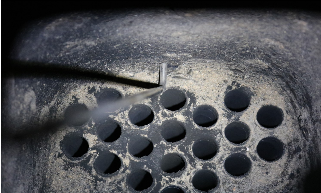
Image of typical 1:8 scale miniature locomotive boiler firebox tube sheet illustrating placement of end of water level device pipe near to the highest point of fireside of crown sheet.
